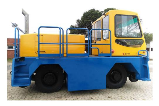
The 'LocoTractor' (LOK) is a highly versatile diesel road/rail vehicle suitable for a range of shunting and freight handling situations.
