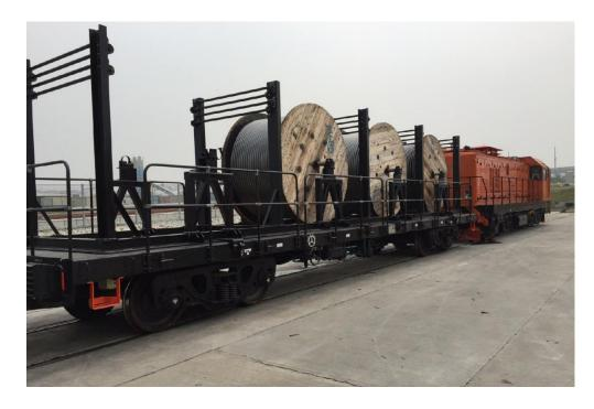
Built 2014 to 2015 by KTK Group China, Romic are pleased to offer for sale 38 of these bogie flat wagons. Ideally suited for freight or infrastructure use; carrying of long / heavy goods such as steel rail, turnouts, poles, transformers or for cable drums for cable laying (power/signal).
